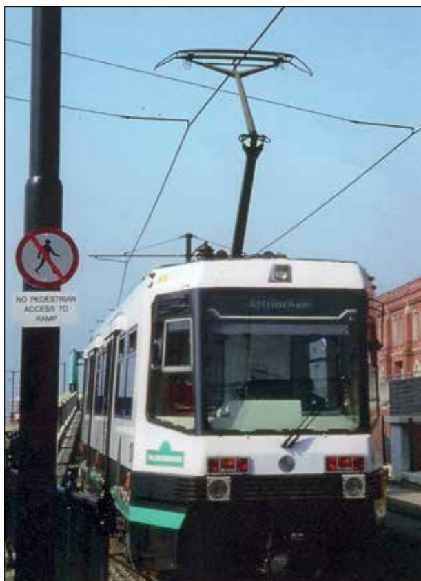
Pull-off made of type A13.5mm parafil synthetic rope with Malico terminals on the Manchester Metrolink.
